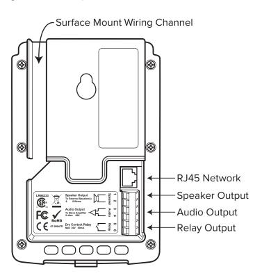
Note: 1. Loudspeaker connects to Speaker Output pins
